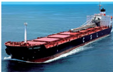
加拿大籍7.4万吨油船“娜丽”轮改装成矿砂自卸船 MT Niles from Canada, a 74,000 DWT Panamax Tanker was converted into self-unloading ore carrier.
