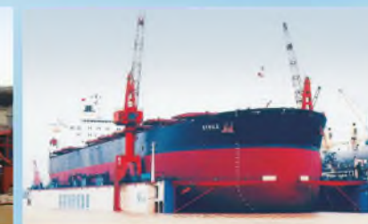
10万吨级“衡山”坞 100,000 DWT Floating Dock: "Heng Shan"
