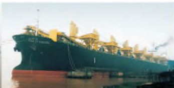
印度籍7.2万吨巴拿马型散货船“迪拜珍珠”轮改装成自卸运煤船 MV Gem of Ennore, a 72,000 DWT Bulk Carrier (ex. Pearl of Dubai) from India was converted into Self-unloading Coal Carrier.
