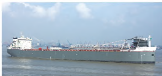
加拿大籍原1.5万吨“莱迪亚”油轮改装成2.5万吨“马尼图林”自卸散货船 M.V. Manitoulin (EX Lalandia Swan), Lake size and Gravity type Self-unloading Bulk Carrier converted from oil tanker.
