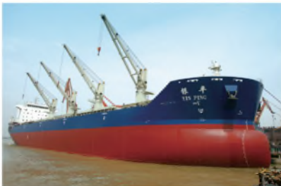
53000吨散货船，中船集团第一艘满足PSPC要求的散货船 The first 53,000DWT bulk carrier adopting PSPC standard within CSSC group was delivered
