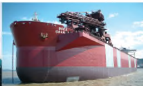
委内瑞拉籍13.5万吨OBO船“波卡”轮改装成矿砂转运平台 MV Boca Grand II, a 135,000DWT OBO from Venezuela was converted into a self-unloading ore transfer station.
